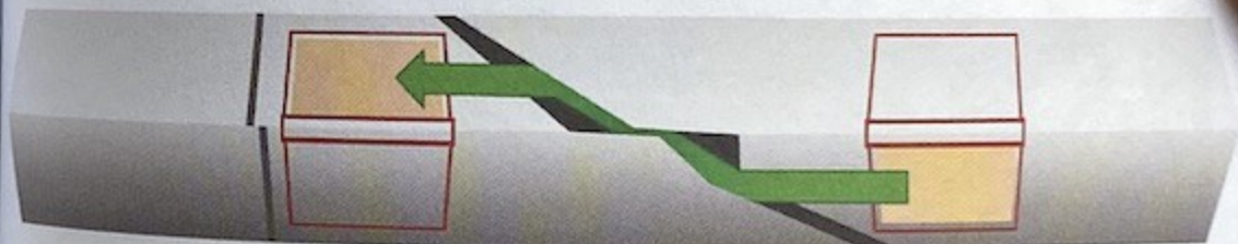
The pages are scanned as they travel across two imaging sensors.
